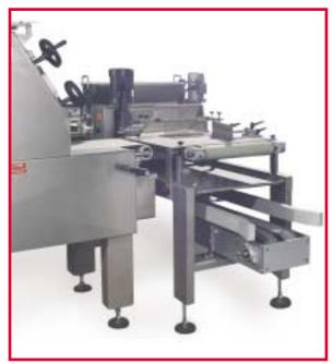
Easily removable endless transfer belt 18" wide. Delrin transfer plate and stainless steel adjustable plow. D.C. removable stainless steel rotary flour sifters.
